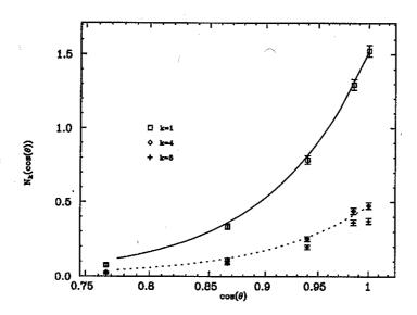
FIG. 2. Number of triggers as a function of arrival angle and k for photons of 100 GeV. Also shown are the  $\cos(\theta)^{\alpha}$  fit.
