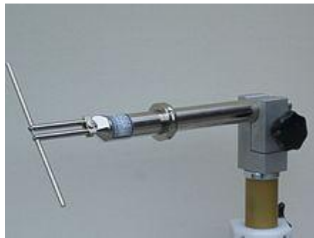
Figure 4. Typical UHF center-fed half-wave dipole antenna . [4]
