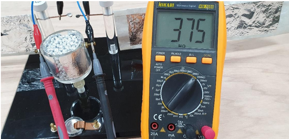
Figure (1.6a). Coherer resistance before the spark in the emitter (375 MΩ)
