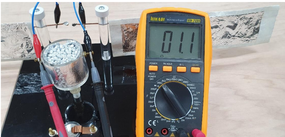
Figure (1.6b). Resistance after the spark in the emitter (1.1 Ω)
