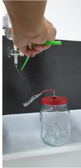
Figure (A.2). Photo showing charged droplets being collected by the electroscop.
