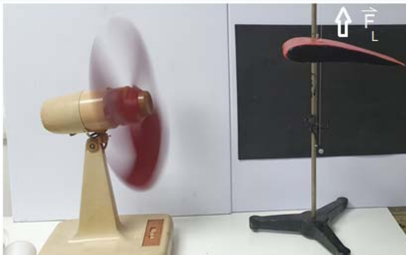
Figure (C.5b). Fan is on and wing suspended by the lift force F_L .
