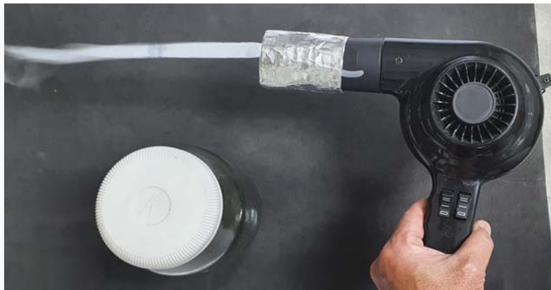
Figure (A.2). The airflow passing far from the cylinder.
