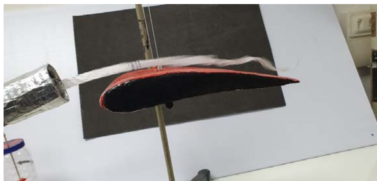
Figure (C.2). Air flow passing near the top of the wing.
