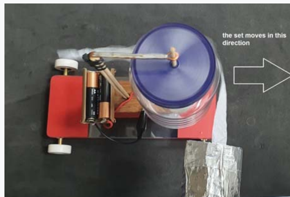
Figure (D.3). Cylindrical pot rotating in anti-horary sense and air flow close to the cylinder. In these conditions, due to Magnus force, cart moves forward.
