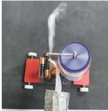
Figure (D.2). Motor on and pot rotating in the anti-horary sense. Air is deflected.
