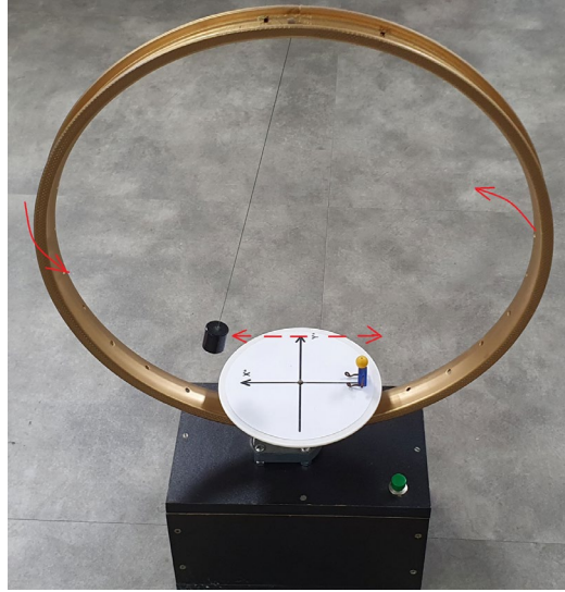
Figure (4.3). Pendulum and circular support positions after 180° angular rotation of the platform.
