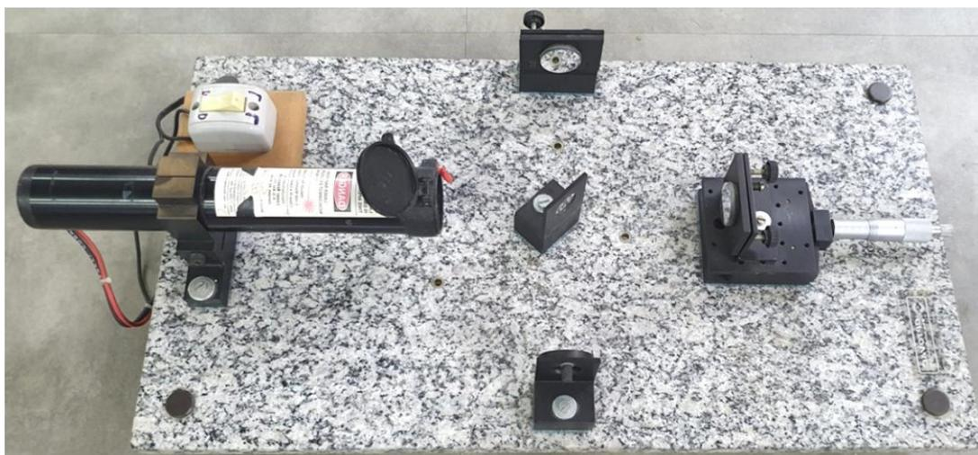
**Figure(2.3).**Small Michelson interferometer of our didactical laboratory.
