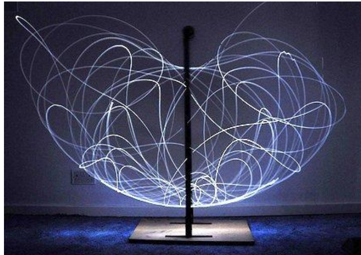
Figure (3.3). Trajectories of the end point of the double pendulum.
