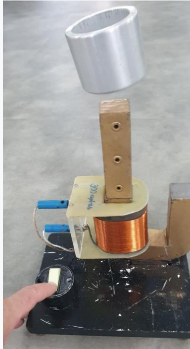
Figure (C.2). Instantaneous repulsive magnetic force on the ring.
