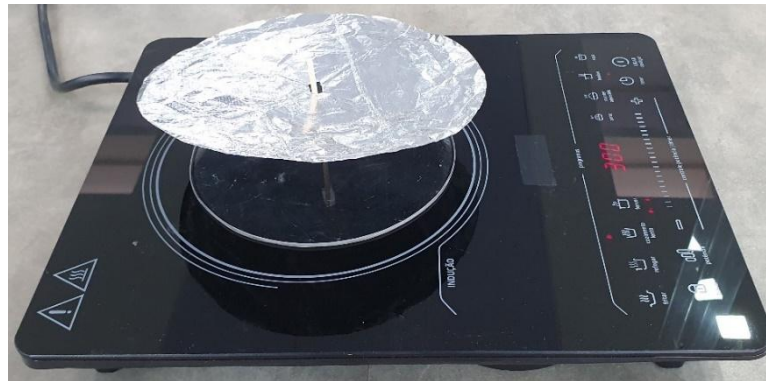
Figure (D.4.c). Aluminum foil levitating over the induction oven on.
