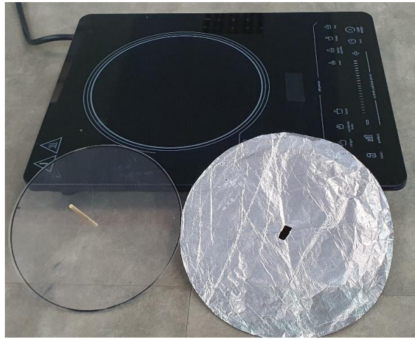
Figure (D.4.a) Induction oven, aluminum plate (kitchen aluminum foil) and a plastic holder with wooden pin.
