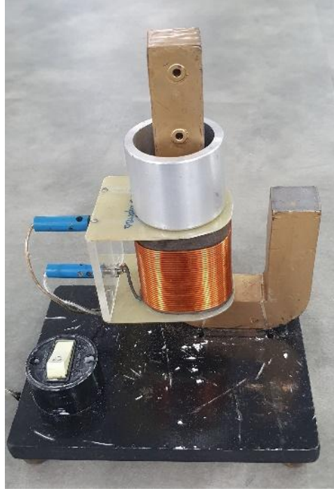
Figure (C.1). Aluminum ring at rest over a solenoid at our laboratory.
