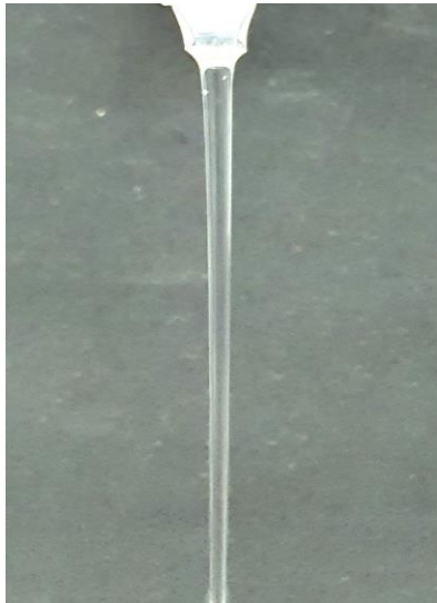
Figure (2.1). Initial laminar flow of mass elements during the free vertical fall.
