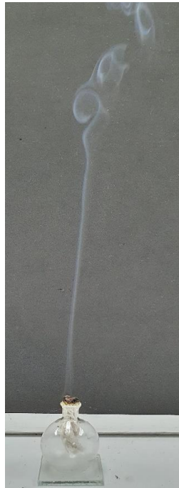
Figure (B.2). Candle flame flow. The low part is laminar and the upper is turbulent.
