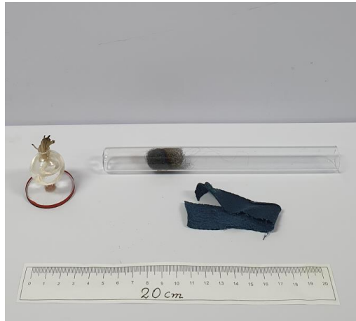
Figure (3B.1). Alcohol container, glass tube with iron gauze and humid cloth.
