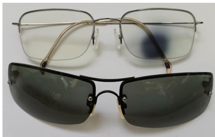
Figure 9. We observe that Photochromic lens becomes darkened by radiation that passed through the sunglasses.
