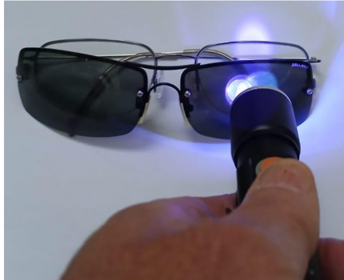
Figure 8. Dark sunglasses between the flashlight and the photochromic lens.
