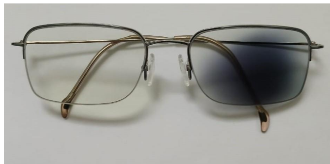
Figure 6. Right lens darkened after exposure to UV-A radiation.
