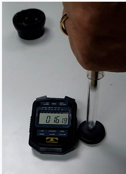
Figure (3.4a). At the initial instant of compression L_i = 120 mm.
